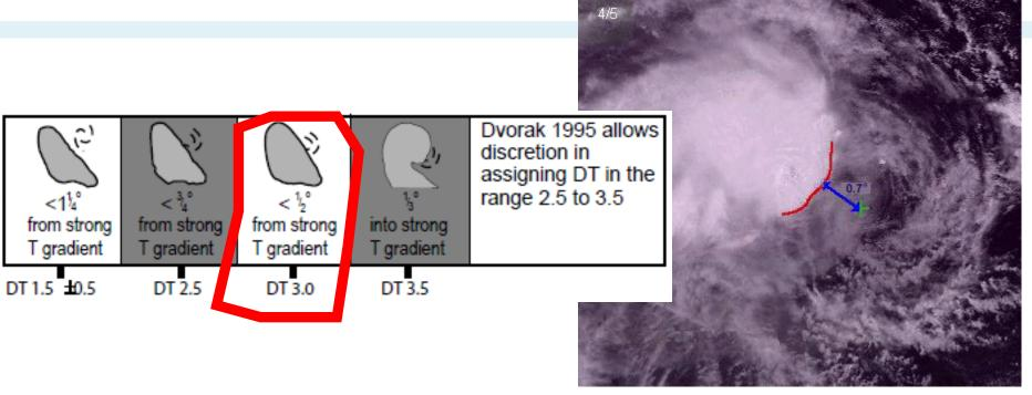
Method: Measure the distance form the low level centre to the edge of the "dense overcast"
