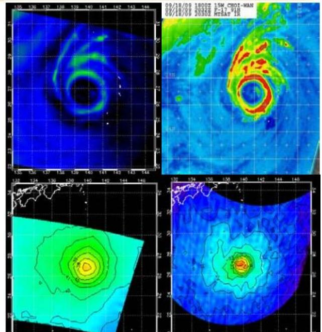
SSMIS Channel 5 Tb Anomalies Compared to Aircraft-Measured MSLP Anomalies
